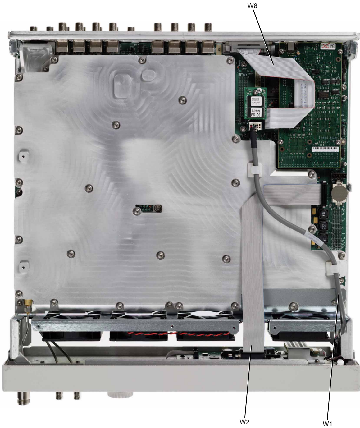
Figure 3-4 Cables from a Bottom View
